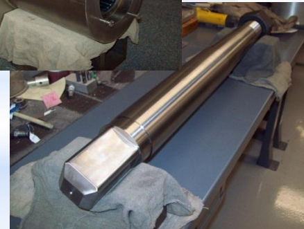
Bearing housing and Drive Shaft (right)
