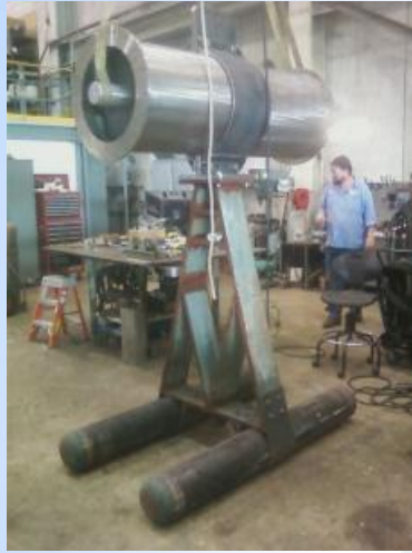
Frame and ballast weights after priming (below)
