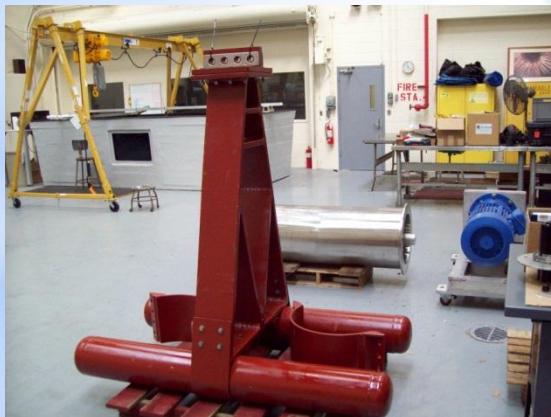
Frame and ballast weights after priming (below)
